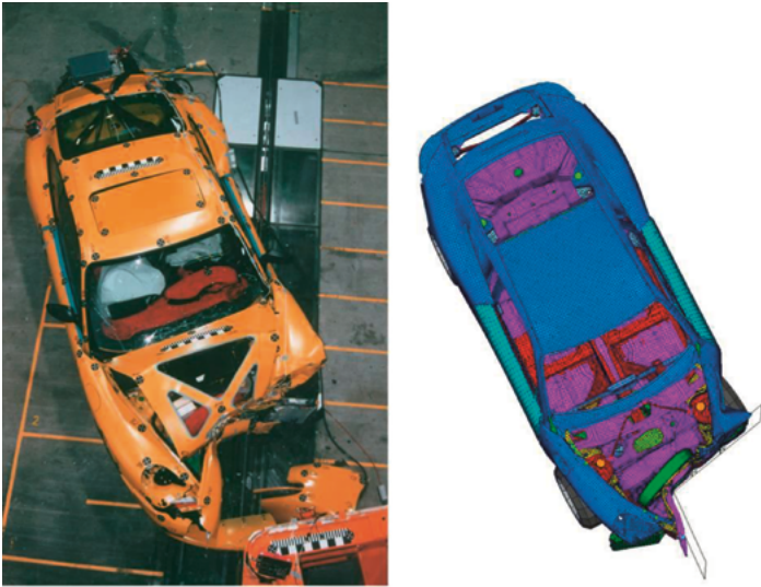
Fig. 5: Crash and simulation in the 1990s: a Porsche 911 Carrera after a frontal offset collision.
